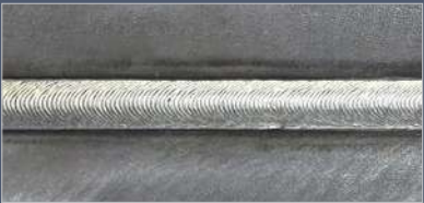
Front side welding form
