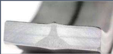
Cross section welding form
