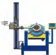
Pipe-flange internal fillet welding
