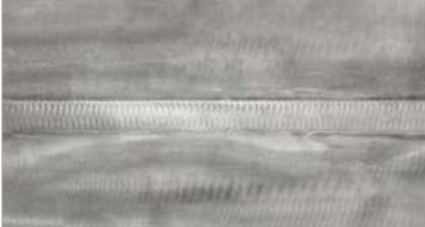
Front side welding form
