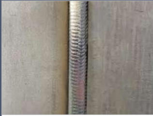
Cylinder longitudinal seam PAW welding
